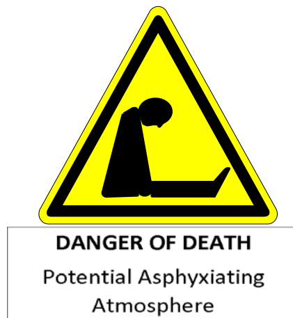
Figure 1—Example of a warning sign for asphyxiation hazard
