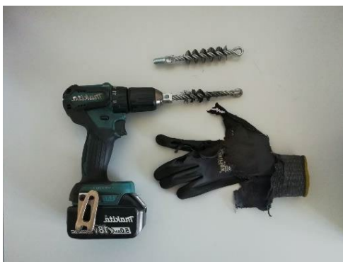
Fig. 3 Cleaning of Cylinder Neck Thread
