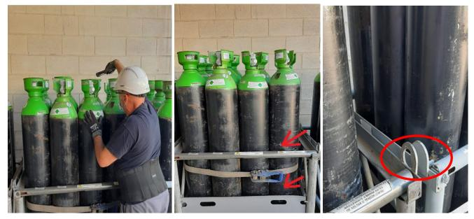
This is not an uncommon event but illustrates that even with everyday tasks, consideration for personal safety is always required. In this case a poor decision by the operator to use an easy but unsafe access method resulted in a fall from height.
