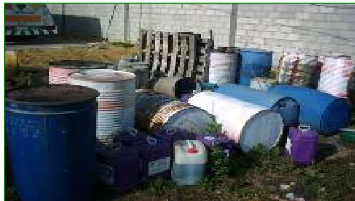
Figure 2 Drums stored outside of containment
