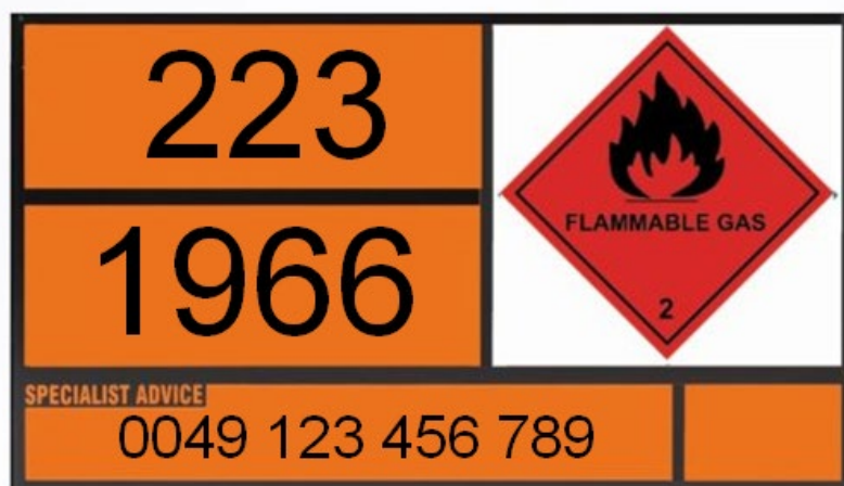
Figure 9: Example of placarding for Cryogenic Liquid H 2 223: Hazard identification: refrigerated liquified gas, flammable 1966 : Hydrogen, Refrigerated liquid
