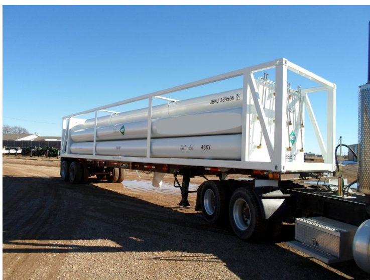
Figure 7: MEGC –demountable from chassis
