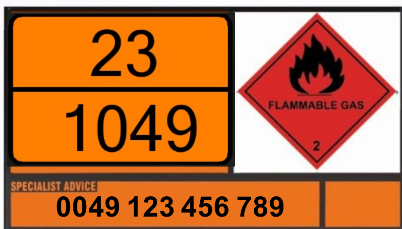
Figure 8: Example of placarding for Gaseous Compressed H 2 23: Hazard identification: Flammable Gas 1049 : Hydrogen, compressed
