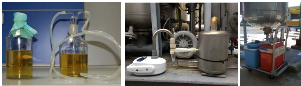
Figure 1-2-3: images of different sampling apparatus: bubbling, cyclone and impaction [12].
