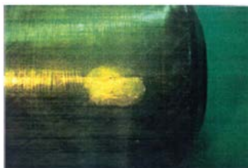
Figure 3: Level 3 impact damage from EN ISO 11623, with depth of damage over 15% of thickness.
