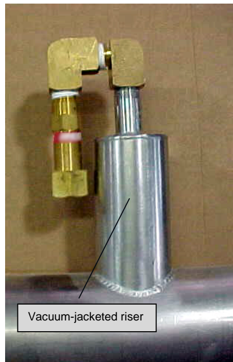
Figure 8 Example of a vacuum jacketed riser
