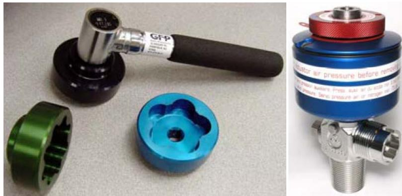
**Figure 4 Typical handwheel torque wrench and an air actuated valve with a DISS outlet**
