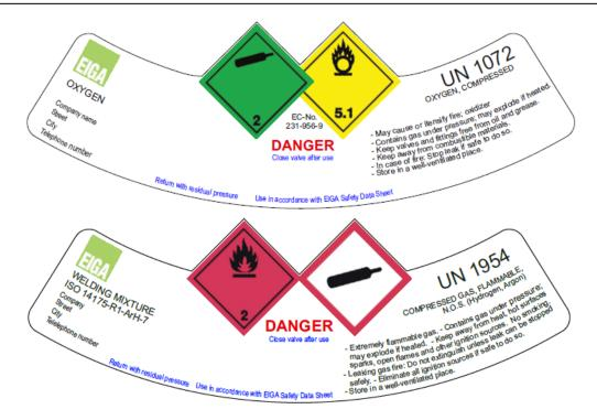
6.6.2 With a shoulder label and a body label for a pure gas (where the CLP symbols identical to the transport symbols have been omitted on the body label
