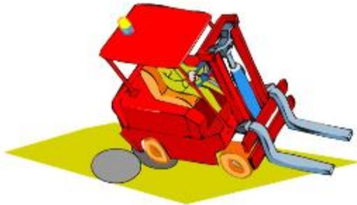
Figure 9 Illustration of FLT starting to turn over
