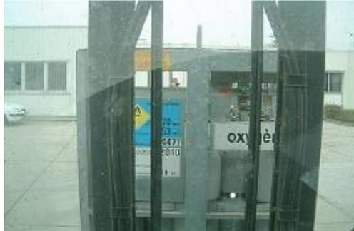
**Figure 13 Example of visibility reduced by when carrying a bundle of cylinders**
