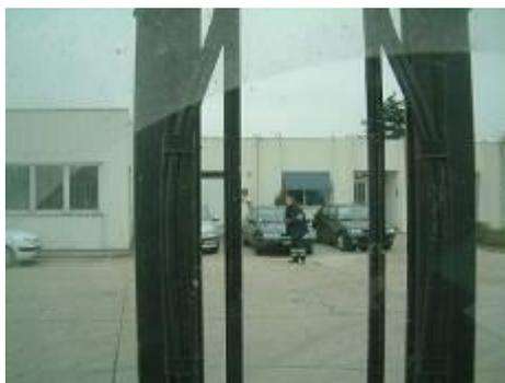
**Figure 12 Example of visibility reduced by FLT mast**
