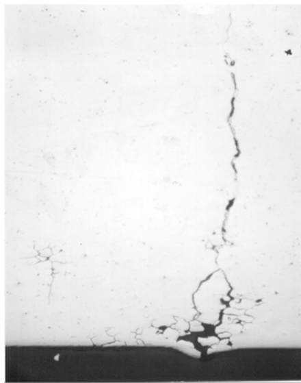
Figure 1—Hoop-wrapped cylinders (AA6061) fatigue crack initiated from a corrosion pit (Magnification x125)
