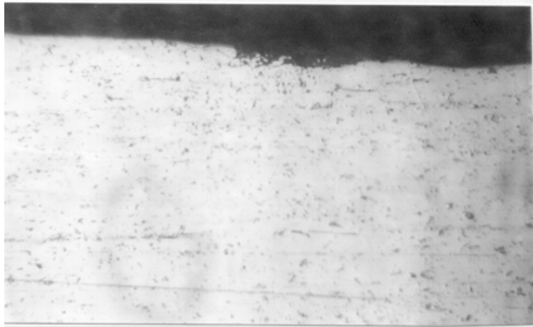
Figure 2—AA7060 Cylinder metallographic examination according to the intergranular test as per ISO 7866 (Magnification x 300)
