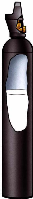
**Figure 2: Cylinders for discharging gaseous carbon dioxide**
