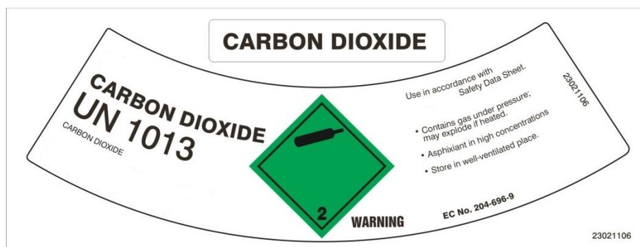
Figure 1: Typical cylinder label
