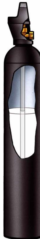
**Figure 3: Cylinders for discharging liquid carbon dioxide**
