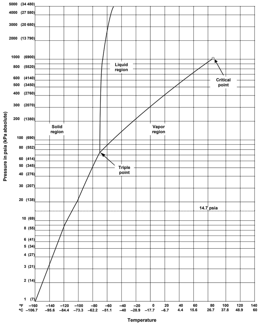
Figure 1 – P-T Diagram of carbon dioxide
