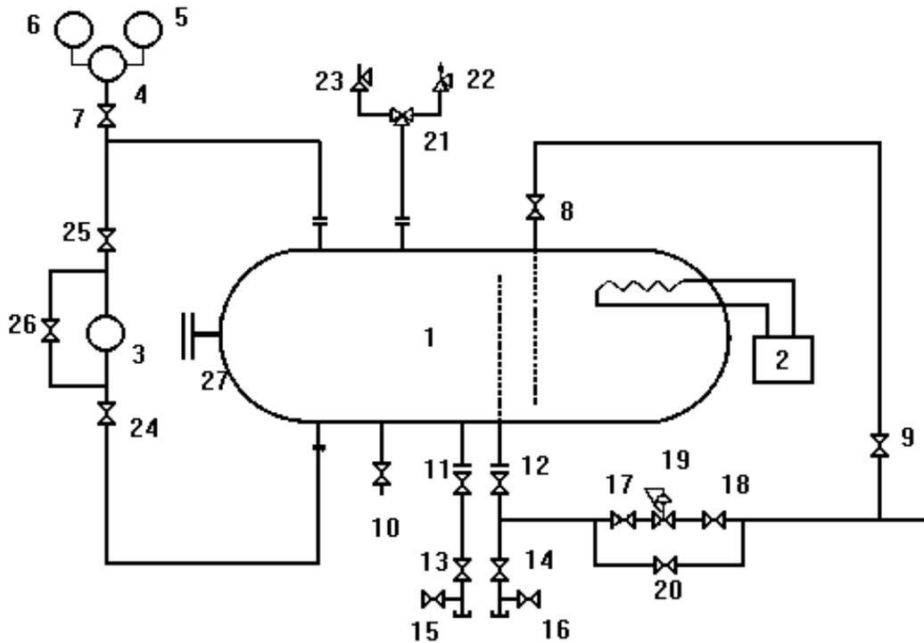
Figure 2 – Example of a non-vacuum insulated storage tank
