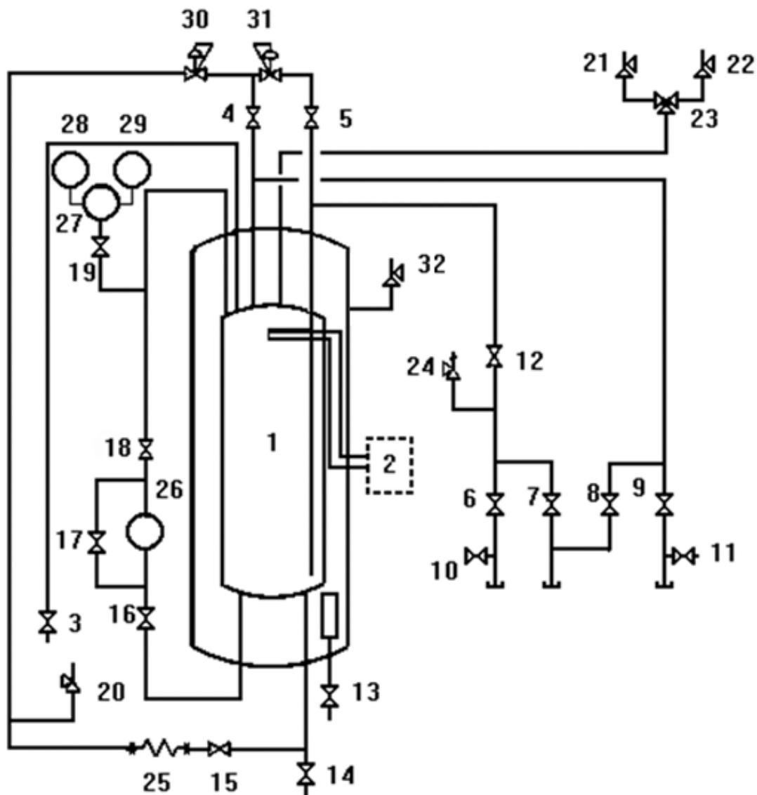
Figure 4 – Example of a vacuum insulated storage tank
