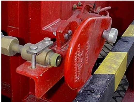
Figure B-1: Tow-away incident prevention device blocking the coupling when activated
