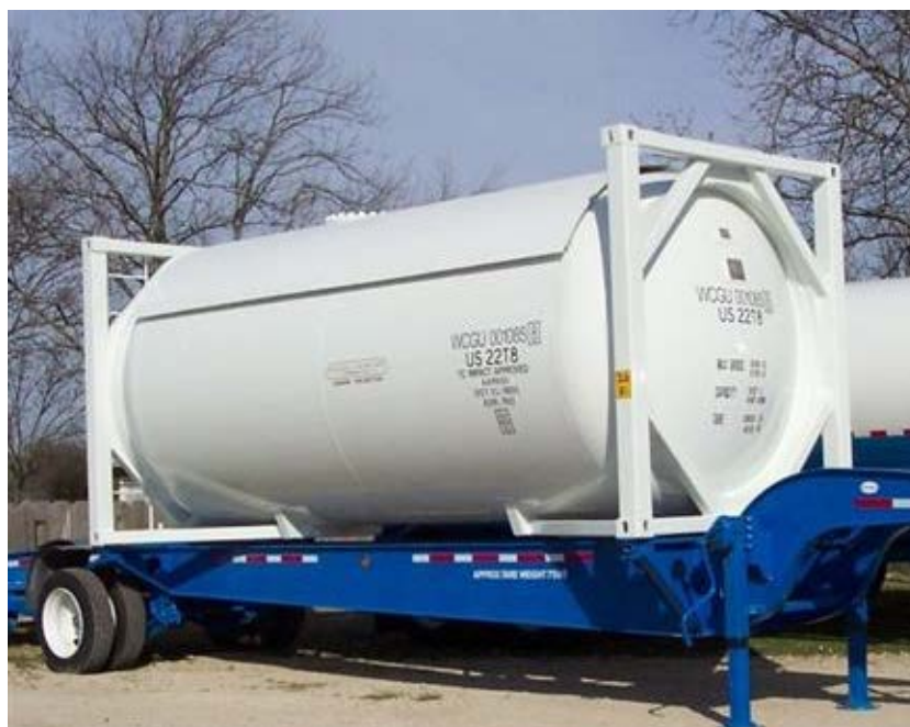
Figure A-4—Portable tank for liquefied gas (20 ft non-insulated container with sunshield)
